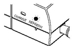
When the battery pack is completely discharged, the CHARGE light begins blinking as the battery pack automatically starts recharging.
